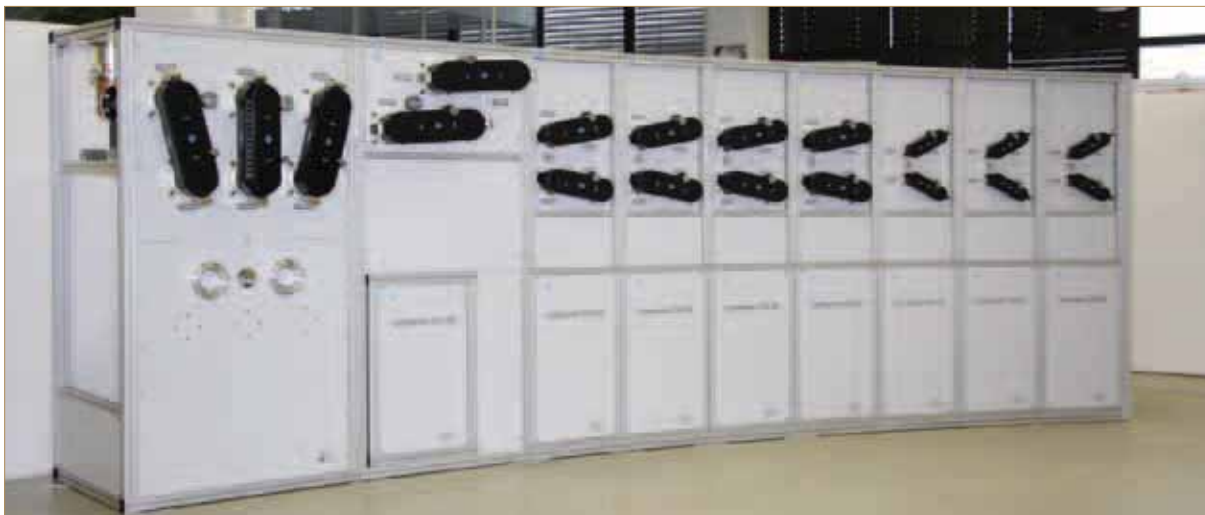
BN 57 53 06 Turkmenistan UHF combiner for 8 x 4 kW DVB with integrated mask filters, combiner bypass and antenna patch panel with bent front for installation in circular transmitter hall
