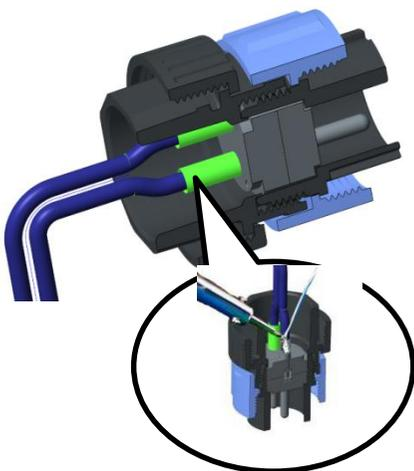
4. Tighten the backshell and compression nut according to the torque.
