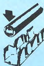
1. Prior to conductor insertion.
