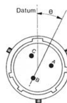
Alternative position of insert with pin contacts (Ø clockwise)
