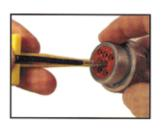
3. Pull contact/wire assembly out of conector. **NOTE:** Do not twist tool or insert at an angle.
