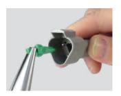
**Step 1:** Remove green wedge using needlenose pliers to pull wedge straight out.
