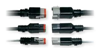
The DEUTSCH DT and DTM Series backshells are designed to snap onto and mate with all standard (basic plug and receptacles without modifications that affect the rear of the connector) DT and DTM Series connectors. The rigid, durable backshells offer a high level of protection and allow convoluted tubing to nest within the rear of the backshell. Straight (180°) and right angle (90°) versions and backshells with strain relief for jacketed cable are also available.
