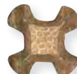
Indenter Crimp Cross-Section Across Axis
