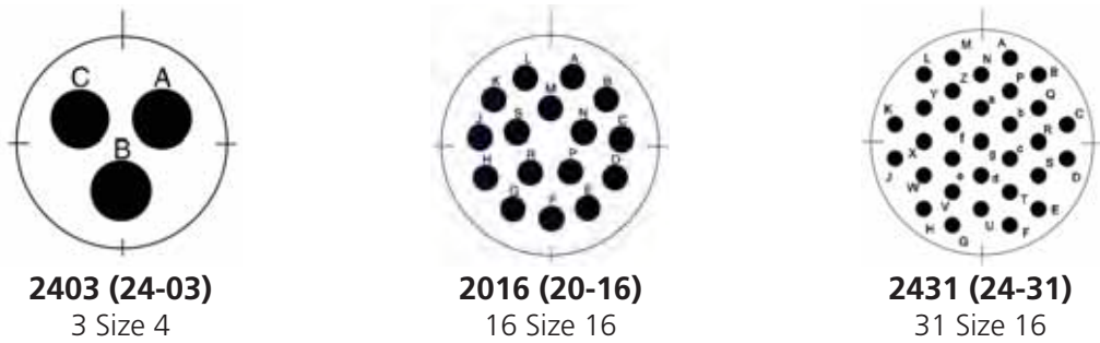
Cavity identification shown from rear socket side
