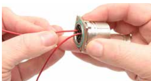
Step 3 - Push contact into place
