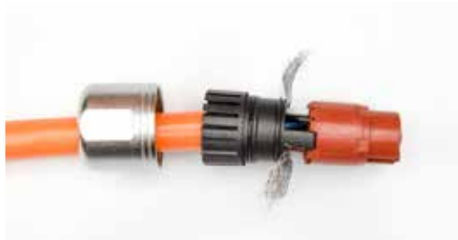
Step 13 - Clip the cord grip as shown with the shield sticking out around it
