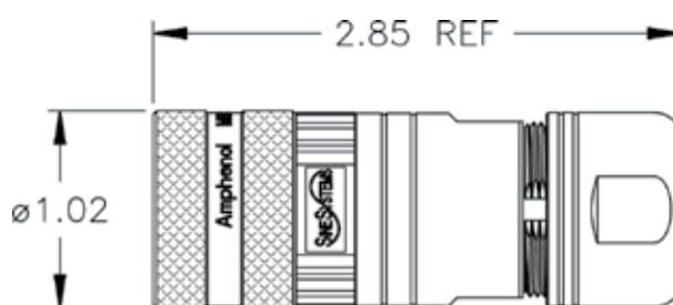
Plug kit straight, threaded; 7.5-11.0mm cord grip
