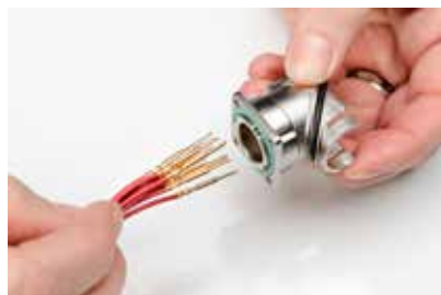
Step 3 - Slide wires through shell
