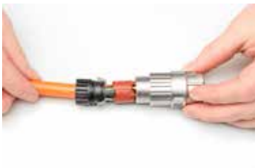
Step 15 - Push sub-assembly into shell
