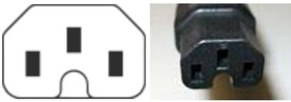
Some electric kettles and similar hot household appliances like home stills use a supply cord with a C15 connector, and a matching C16 inlet on the appliance; their temperature rating is 120 °C rather than the 70 °C of the similar C13/C14 combination. The official designation in Europe for the C15/C16 coupler is a 'hot condition' coupler.
