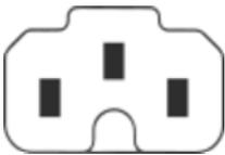
There is also a C15A/C16A coupler, with an even higher (155 °C) temperature rating.
