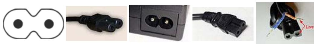
Commonly known as a *figure-8* or *shotgun* connector due to the shape of its cross-section. It is also known as a *euro-connector* in electronic shops. A polarized C7 (C7-PW) used to exist, but is not part of the standard, it was asymmetrical, with one side rounded (neutral) and the other side squared off (line).
