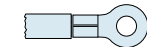
Small Ring for Attaching Receptacle Covers to a Panel with a Screw
