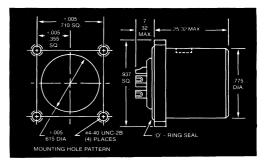
Barrel Pin Terminals\* Mates with U-183/U, U-228/U & GC 183S GC 429 Receptacle Rigid Contacts
