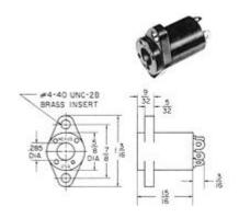
**Flanged Rear-Mounted Jack**Mates with NEXUS Series TP-120 plugs and plugs TP-101 and TP-102. Nickel plated beryllium contacts are anchored in a phenolic body.
