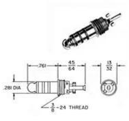
Threaded Telephone Plug Mates with NEXUS series TJ-120 and TJ-102 jacks and jack TJ-101. For custom molding directly to cable. Same as TP-120-7 but strain relief clip omitted.
