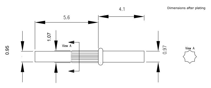
NOTE 1 :- For use in finished board holes measuring 1.02 ±.010 per industry standard
