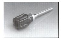
This terminal has an easy grip, captive head containing a 4mm socket. It has a 2.1mm diameter crosshole in the clamping gap which is free from threads.
