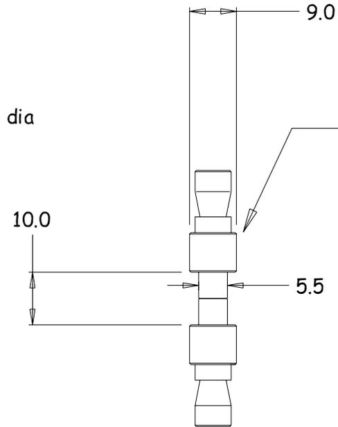
All external edges corners and radii chamfered 0.1mm
