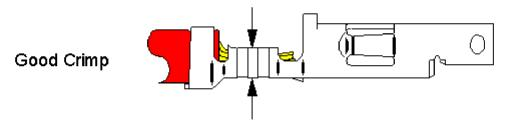
Solution: Verify Correct Terminal for AWG or Adjust Conductor Crimp Height on Press
