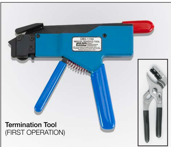
Roll Over Tool (SECOND OPERATION)
