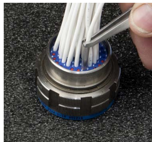
Typical All Metal Tool Operation
