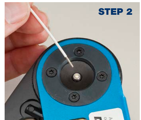
INSERT PRE-STRIPPED WIRE
