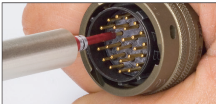
Typical application showing tool testing pin contacts.
