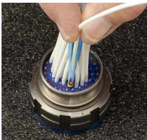
Typical All Plastic Tool Operation
