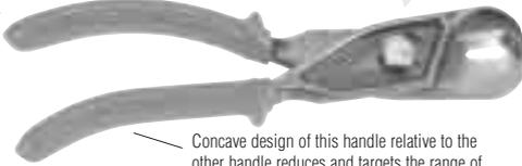
Concave design of this handle relative to the other handle reduces and targets the range of motion where the hand and forearm have maximum leverage.
