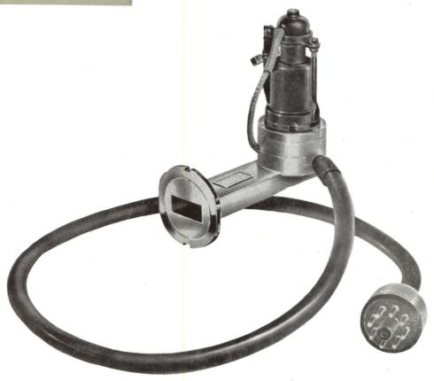
This component consists of a short-circuited section of waveguide size 16 fitted with a mount to support a valve base which is wired for use with klystron type 723 AB. (CV 1795). Connections from the base are brought out into a 3 ft. length of cable, which is terminated with an octal plug.
