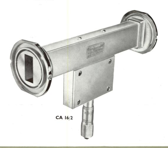
A micrometer is coupled via an antibacklash system and two rods extending through the narrow wall of a waveguide to a metallised glass vane in the guide. This provides a mechanical discrimination of the position of the glass vane to better than 0.1 db over the range 0 to 40 db.
