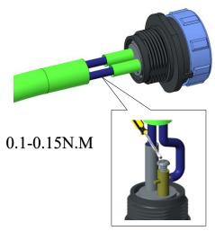
3.Put the socket through the panel cut hole.
