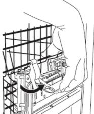
Fig. 7 Adjusting the upper rack for DW60CD models
