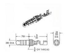
**Threaded Telephone Plug**Mates with NEXUS series TJ-120 and TJ-102 jacks and jack TJ-101. For custom molding directly to cable. Same as TP-120 but without plastic shell.
