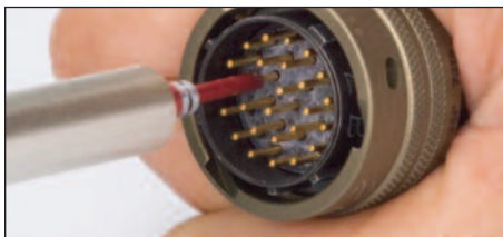
Typical application showing tool testing pin contacts.
