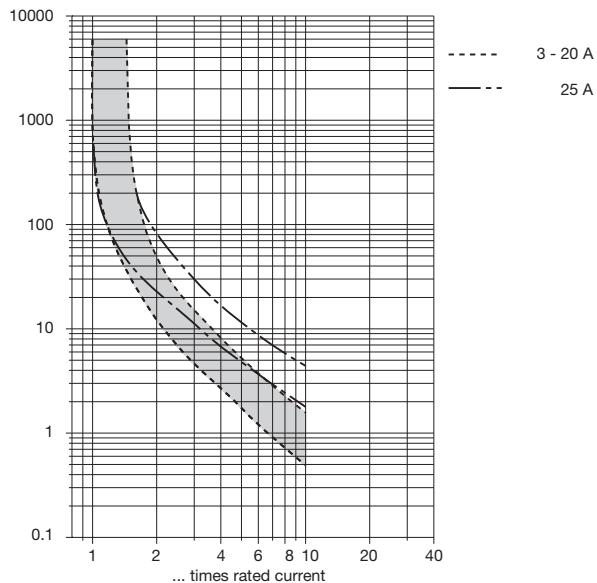
The time/current characteristic curve depends on the ambient temperature prevailing. In order to eliminate nuisance tripping, please multiply the circuit breaker current ratings by the derating factor shown below. See also section 9 – Technical information.
