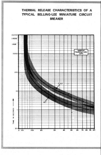
The L5200 series operates thermally on moderate over-currents, but with large fault currents (above 6 to 10 times the rated current) a magnetic coil takes charge, tripping the mechanism virtually instantaneously, i.e. in a matter of milli-seconds. This series of circuit breakers meets the majority of requirements.
