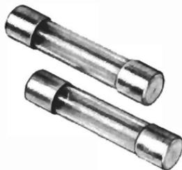
These standard glass fuse links are for protection of telecommunications and light electrical equipment. They have a minimum life of 1,000 hours continuous rated current at 25 °C. They blow within 10 seconds at 2 x In (+ 20% to -0%). The derating for operation at elevated temperatures is: 1,75% per 10 °C up to 100 °C.
