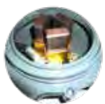
B - Earth Return Current units - Carbon brushes
