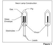
material known as dumet which is a low resistance material consisting of a copper sheath around a nickel iron core constructed so that its expansion coefficient is the same as that of the glass used for the bulb. Butt welded to the lead wires are nickel electrodes of larger
