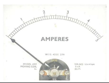
The simple formula for calculating the required currentshunt resistance RS (Ohms) to enable a meter with a fullscale sensitivity of Im (Amps) and internal resistance Rm (Ohms) to measure Ifs (Amps) is:
