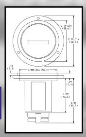
Three-Screw Mount: Panel cut out 2.00 diameter opening. Three .125 holes equaly spaced on 2.42 bolt circle diameter.\*
