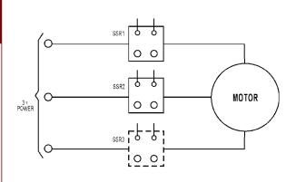
Three-phase motors may be controlled by solid-state relays as shown. A third SSR as shown is optional, but not necessary. The control windings may be connected in series or parallel. Care should be taken to ensure that the surge current drawn by the motor does not exceed the surge current rating of the SSR.
