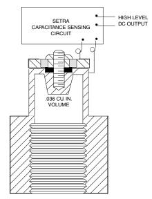
Extremely low hysteresis and very stable operation under extreme temperature conditions are inherent in this sensor design.
