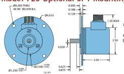
The optional 5PY adapter is made of all aluminum construction and allows Model 725 encoder to replace DC tachometer technology. The 5PY adapter is mechanically interchangeable with any 5PY tach generator.
