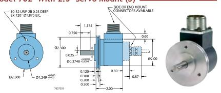
All dimensions are in inches with a tolerance of +0.005" or +0.01" unless otherwise specified
