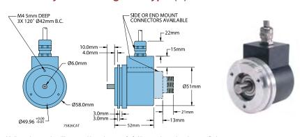
All dimensions are in millimeters with a tolerance of  $\pm 0.17$  mm unless otherwise specified
