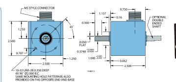
All dimensions are in inches with a tolerance of  $\pm 0.005$ " or  $\pm 0.01$ " unless otherwise specified
