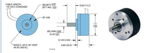
All dimensions are in inches with a tolerance of ±0.005" or ±0.01" unless otherwise specified Metric dimensions are given in brackets [mm]
