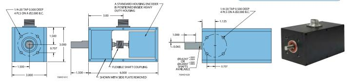
All dimensions are in inches with a tolerance of  $\pm 0.005$ " or  $\pm 0.01$ " unless otherwise specified
