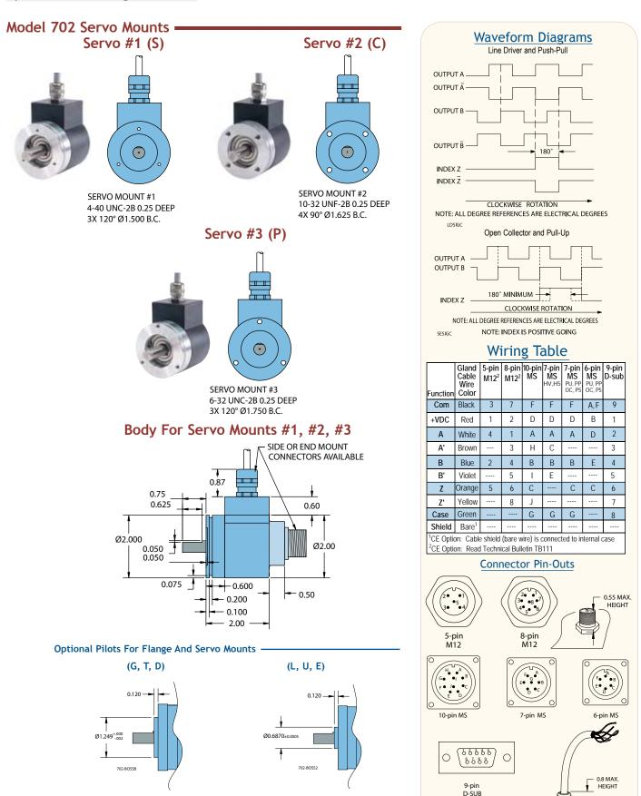
All dimensions are in inches with a tolerance of ±0.005" or ±0.01" unless otherwise specified
