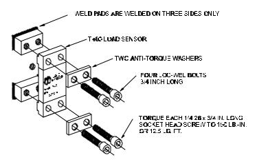
The above illustrations represent the proper arrangement of Model T400 Load Sensor kit parts using either the Drill and Tap method or the Weld method.
