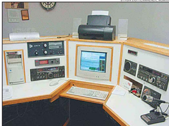
Byron Lichtenwalner, W3WKR, of Stroudsburg, Pennsylvania, searches the bands from this impressive station. It features an ICOM IC-765, PK900 TNC, Alpha amplifier, IBM PC running Writelog and a Mosley PRO-57B at 65 feet on a crankup tower.
