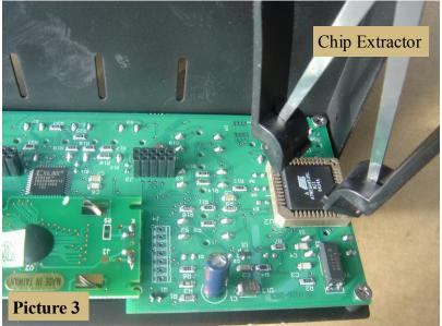
• Using the chip extractor (Picture 2 & 3) carefully pull the CPU chip out of its socket
