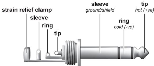
For connection of balanced and unbalanced plugs, ring and sleeve have to be bridged at the stereo plug.
