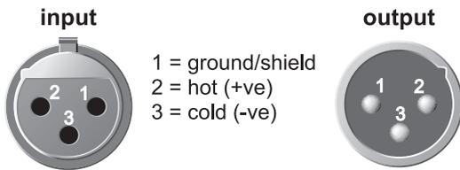
For unbalanced use, pin 1 and pin 3 have to be bridged
