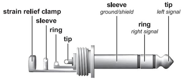
Fig. 3.4: Stereo plug for headphones connection
