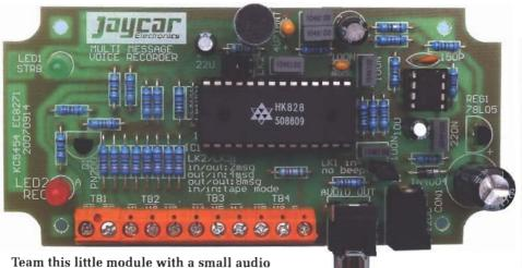
amplifier, to provide a great range of sound effects for a model railway layout, for example. It has the ability to store up to eight different "sound grabs" which could be switched to different parts of the layout as trains pass through stations.
