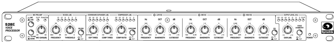
**T**HE 528E IS A COMPLETE, SELF-CONTAINED VOICE PROCESSOR that performs six separate functions: microphone preamplification, de-essing (sibilance removal), compression/limiting, downward expansion, parametric EQ, and voice symmetry alignment. All six processors may be used simultaneously. Although we call the 528E a “Voice Processor”, it is perfectly suitable for any signal, vocal or not.
