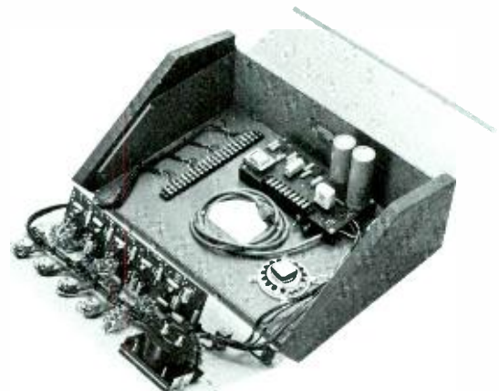
Hinged top cover and front panel give full access to the barrier strips for installation, and all control switches and components for maintenance.
