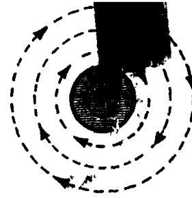
Fig. 3.—THE MAGNETIC FIELD ROUND A CURRENT-CARRYING CONDUCTOR.
