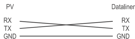
Figure 2.13 PanelView RS-232 Port and Dataliner Connection
