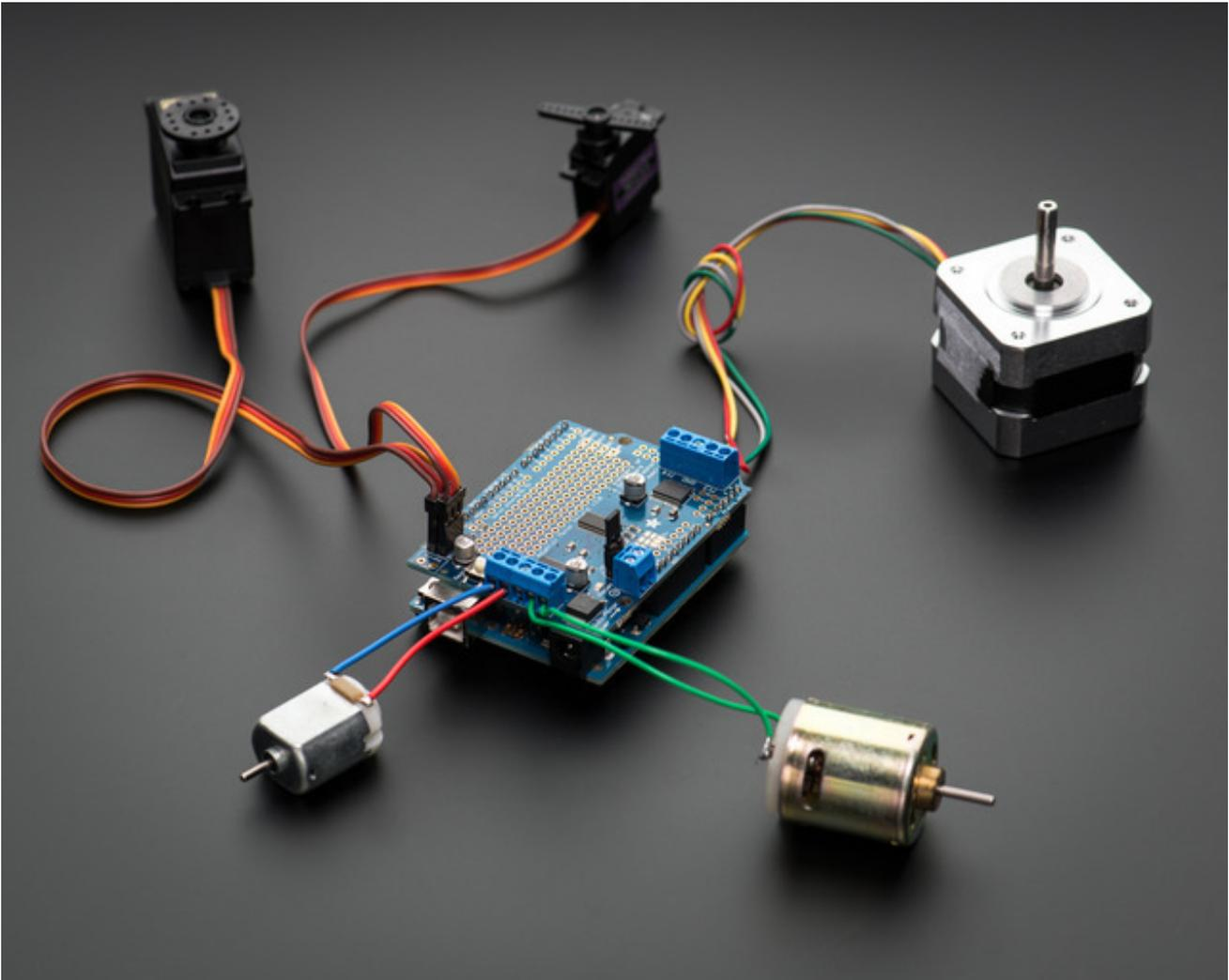
The original Adafruit Motorshield kit is one of our most beloved kits, which is why we decided to make something even better. We have upgraded the shield kit to make the bestest, easiest way to drive DC and Stepper motors. This shield will make quick work of your next robotics project! We kept the ability to drive up to 4 DC motors or 2 stepper motors, but added many improvements:
