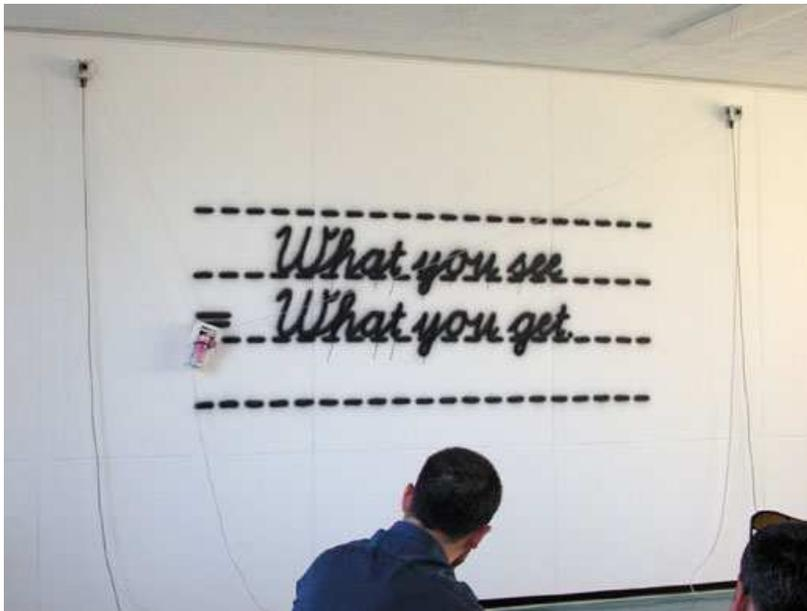
*This is Hektor in action, see <http://www.hektor.ch> for more details and art. The system works by hanging a solenoid operated spray can by two toothed belts that can be fed in and out by steppers. Gravity sorts everything else out.*
