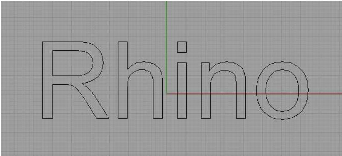
Select the lines and type divide in the command line and accept the seam adjustment. Type L and press return to allow the segment length to be defined and then enter the segment length you want.
