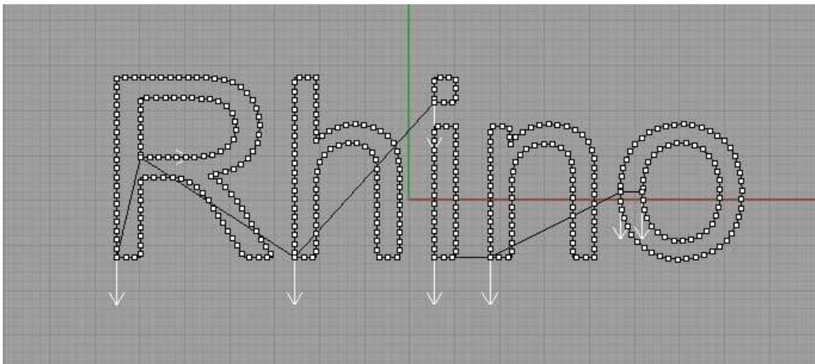
The drawing is now covered in dots that are the distance apart you specified. We will use these to split the drawing into little segments. Type split and when asked for the cutting object select all of the points by dragging a box or type SelPt and press return. Then press return and the lines will be split up
