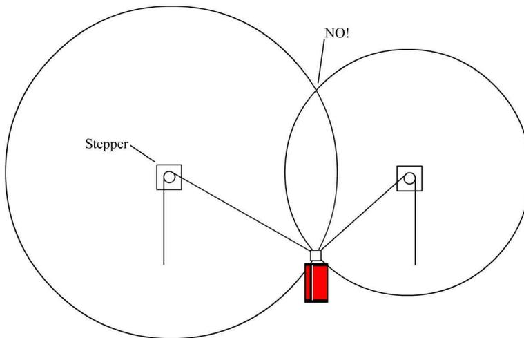
*Hector's struts "force" the spray can to lie on the intersection of two circles but gravity chooses the lower intersection.*
