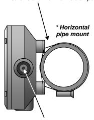
Conduit entries have an integral moulded seal, to remove break seal out using suitable lever (eg. screwdriver or rod)
