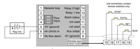
**Wiring requirements:** Use multi-core screened twisted pair instrument cable (0.25~0.5mm²) for electrical connection between the Ecobatch and any flowmeter or remote switch input. The screen needs to be grounded at -0V (terminal 8), this is to protect the transmitted signal from mutual inductive interference.
