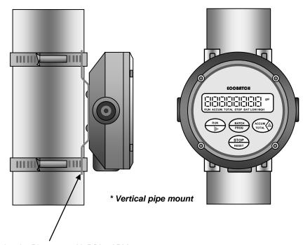
\* order Pipe mount kit P/No. APM comprising two brackets, screws and worm drive clamps.
