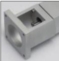
*Optional factory installed motor bracket replaces cartridge end cap. Supports most standard stepper and servo motors in alignment with lead screw. Factory assembly assures correct alignment and sealing integrity.*
