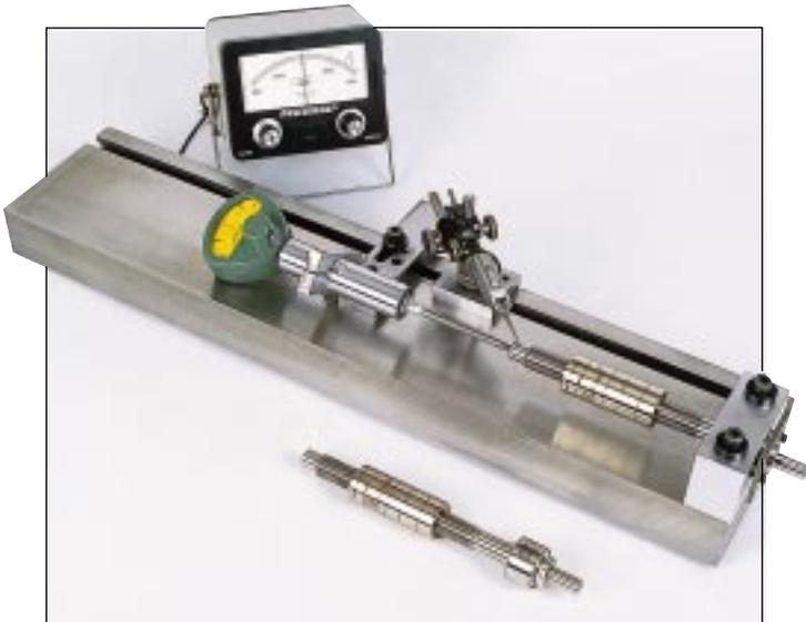
*Inspection of bearing for thrust plane error.*
