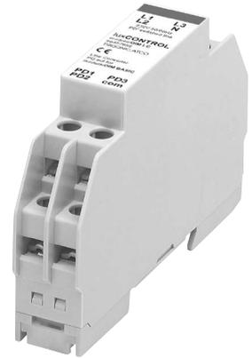
The well known modularDIM system will be extended by the new designed modularDIM LC which provides the opportunity to integrate common, commercial of the shelf mains rated “presence detection (PD) units/sensors” (converts main rated signals into potential free signals based on the galvanic isolation). The modularDIM LC is designed as “to build in unit” for the integration into a switch cabinet. This unit is easy to install
