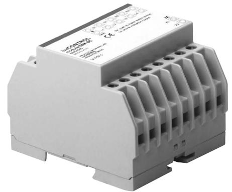
Expansion module for modularDIM systems to control scenes. Enables the recall and programming of four light scenes via the modularDIM BASIC. The switch inputs are SELV and any push to make switches can be used.
