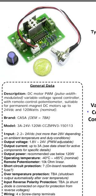
Size: 60 x 44 x 24 mm (nominal LxWxH) Fixing: 4 x M3 clearance holes @ 34 + 50mm (L x W mm) matrix (pitch) Weight: 36 gms
