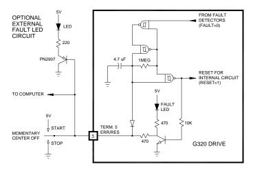
The above circuit shows how to implement an external switch to clear an ERROR condition and RESET the G320, while still being able to read the state of the drive. It also includes an optional FAULT LED circuit if a remote indication of the state of the G320 is desired.
